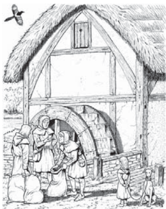
Figure 1-15. Thousands of watermills have been used throughout history as prime movers for grinding grain and powering early machines. Modern water turbines for electric generation and fluid power motors have evolved from these early designs. (©2007 Jupiterimages and its licensors. All rights reserved.)
